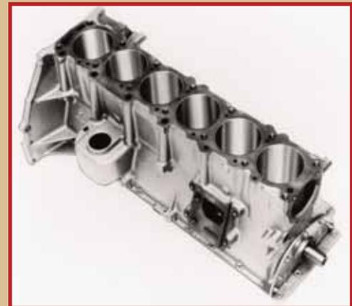
**The Pontiac OHC6 engine was based off Chevrolet's 230ci L-head six cylinder bottom end.**
