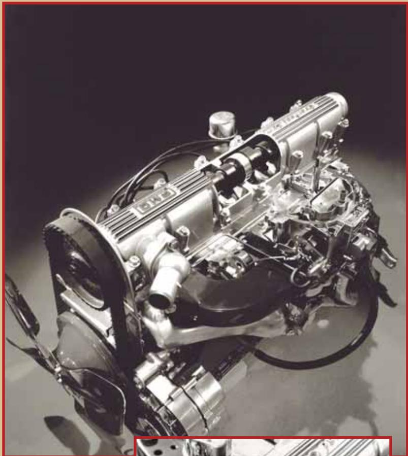
**Cut-away view shows the tall design of this OHC-6 engine and the proximity of the valves to the overhead camshaft. The camshaft was mounted within the cam cover and placed directly atop the valves.**
